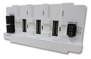
\*LVDS backplane : For I/O module backplane connection LVDS communication cable connection accessory
