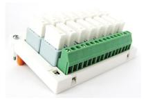
\*Wire holding structure : Screw type
